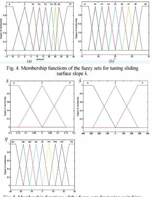
Fig. 5. Membership functions of the fuzzy sets for tuning switching control gain  $\eta$ .
