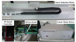
Fig. 6. Photo of the experimental platform
