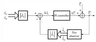
Fig. 2. The inverse secondary time constant estimator.
